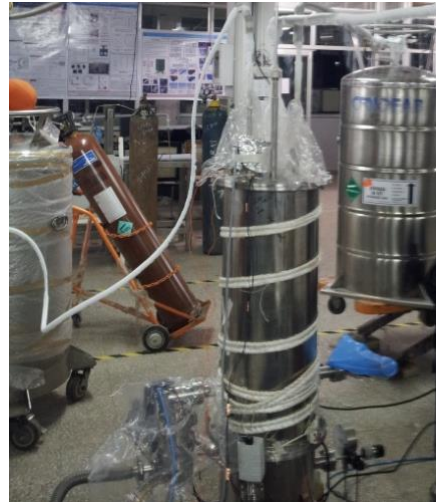
Figure 4: Small Scale Cryo-pumping Facility (SSCF) assembled during pumping speed experiments.
