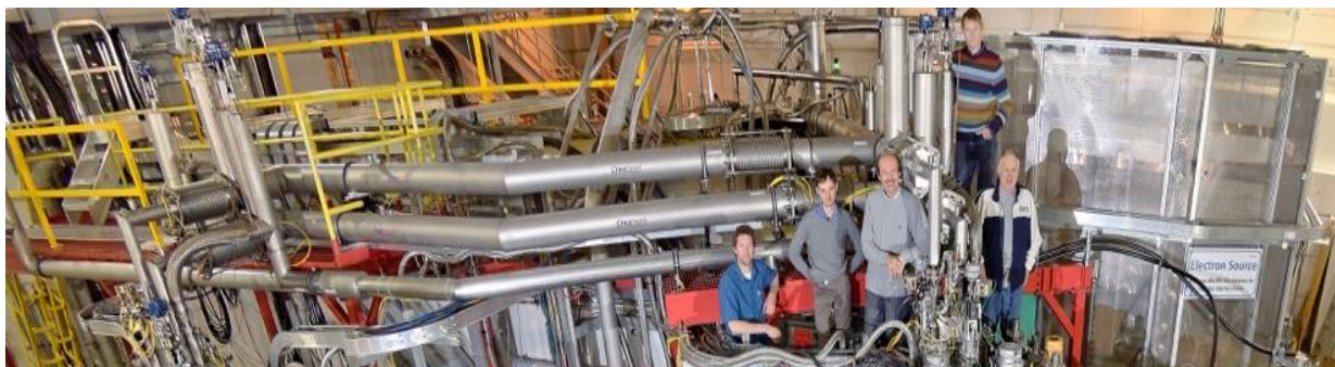
Figure 5. Liquid helium distribution system
