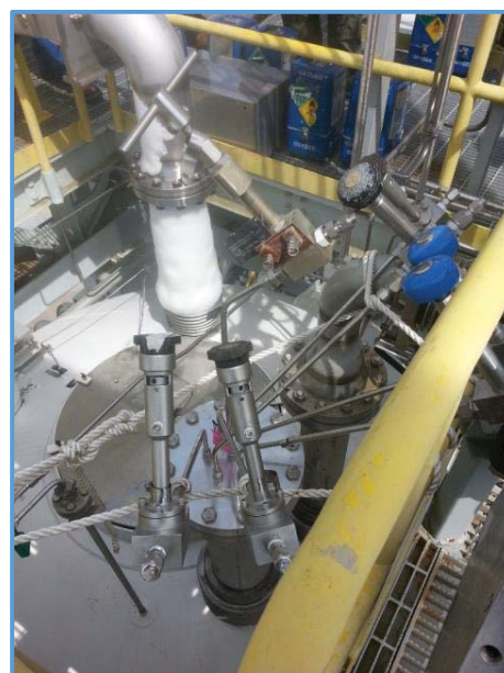
Figure 5. LOX Run Tank Flange Interface/Valves.
