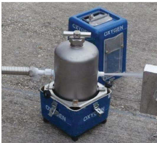
Figure 6. Cosmodyne Cryogenic Sampler.
