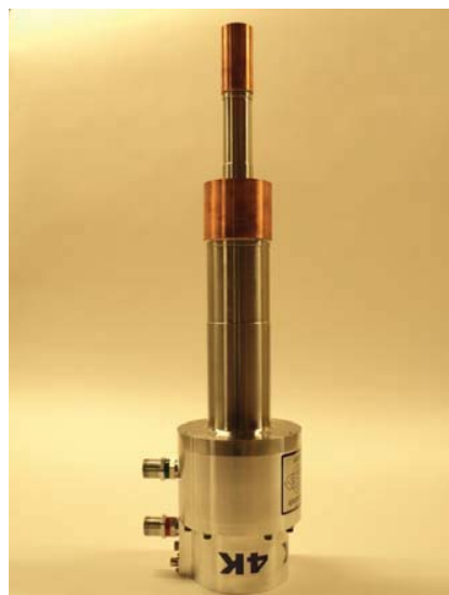
Figure 2. Photo of the pneumatic-drive GM cryocooler (DE215S).
