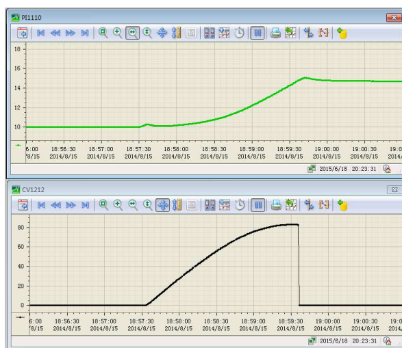
Figure 7. Adjusting effect of high pressure supply when K_p=5.3 , T_i=180 .
