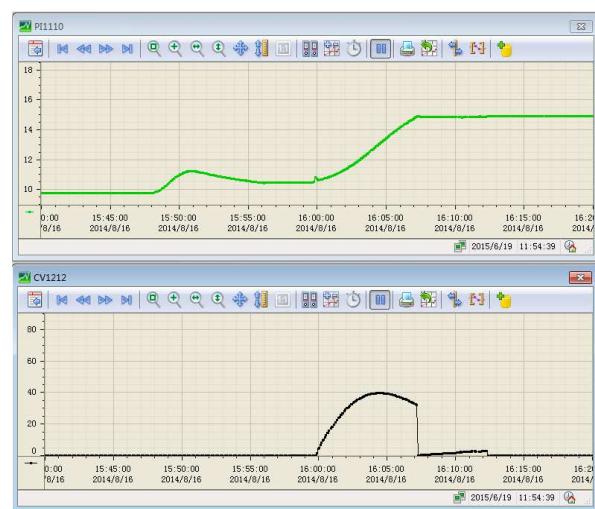
Figure 8. Adjusting effect of high pressure supply when K_p=10 , T_i=3000 .
