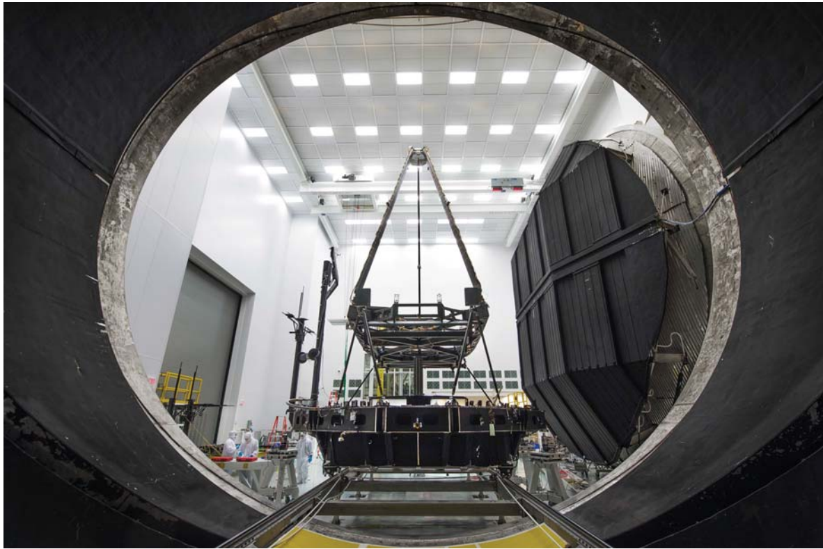
Figure 7. View of the pathfinder structure in the clean room from within Chamber A. This is the next thermal test, which will employ 16 cold radiometers for diagnostics.
