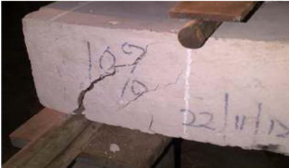
Figure 2. Shear compression failure of a typical beam specimen during flexural test.
