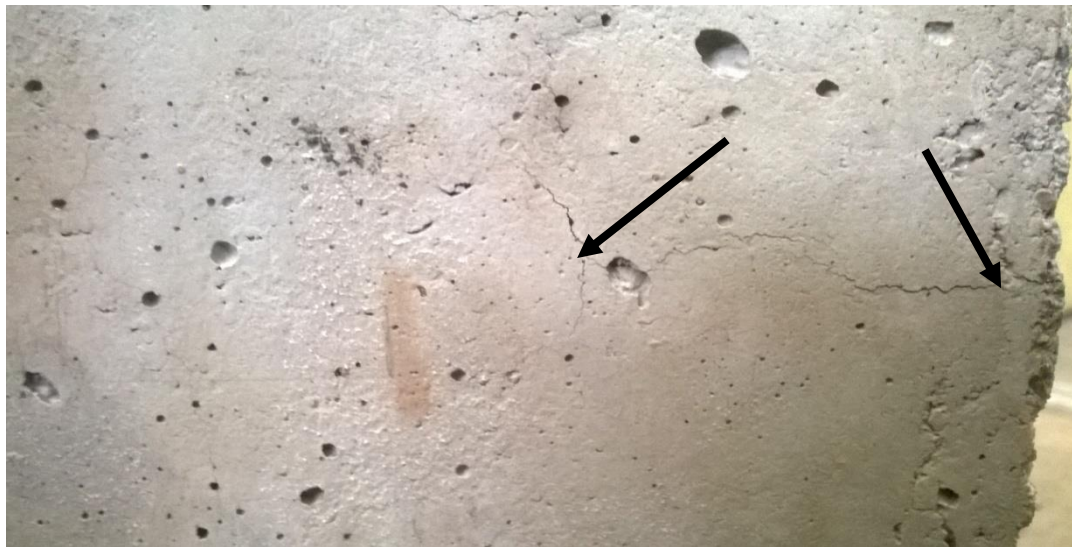
Figure 3. Arrows pointing to crack lines formed on 15% recycled concrete after tempering for 2 hours at 400°C.
