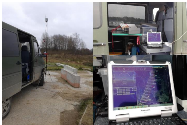
Figure 3. Ground control station used to guide and monitor MUST Q.
