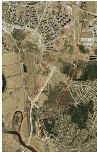
Figure 1. Schematic of partial areal-survey with ground control points of Tartu, concentrating on boroughs of Ihaste and Annelinn.
