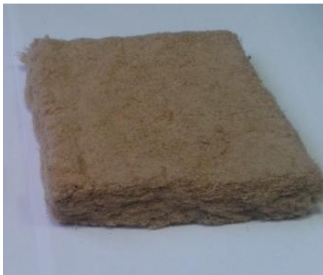
Figure 1. Thermal insulation board from birch fibres.
