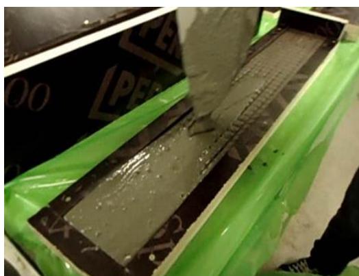
Figure 4. Photography of the RPC being cast with two 2D carbon grids as reinforcement.
