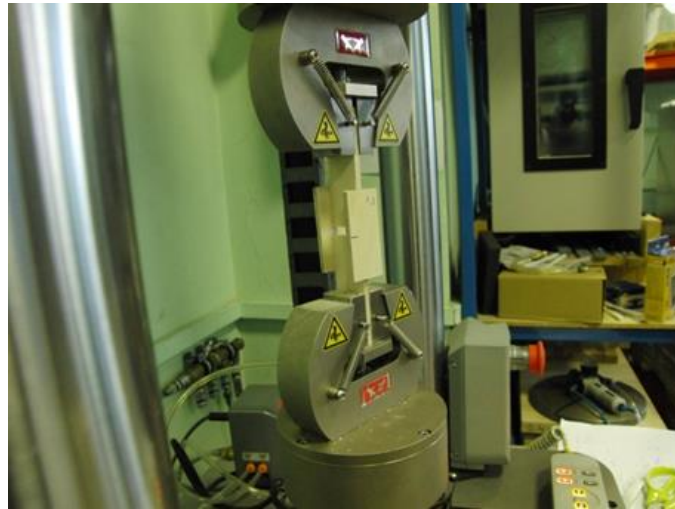
Figure 7. Specimen placed in the testing machine (Instron 3000).
