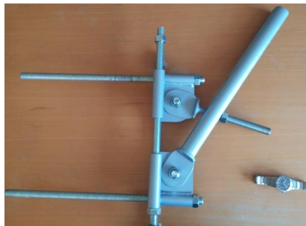
Figure 15. The created optimized Lever Anchor (with the wrist watch in the bottom right corner as a scale).
