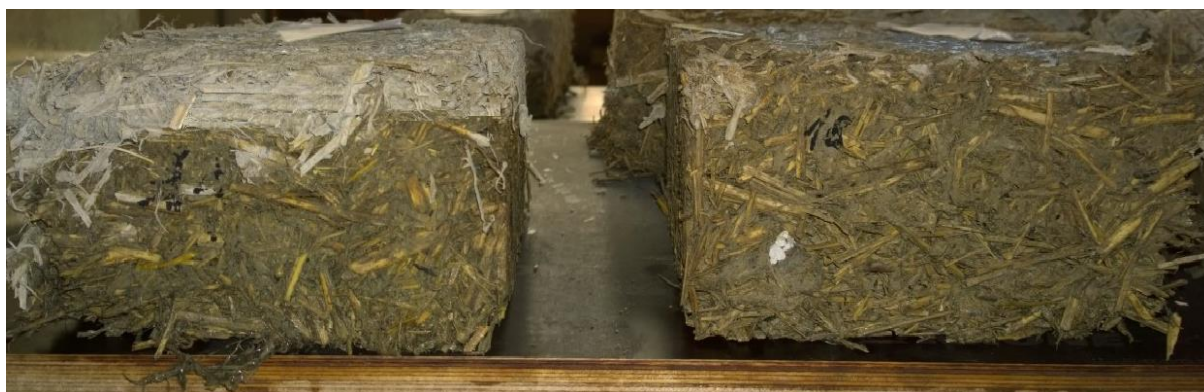
Figure 2. Water absorption test – GCP-W (left) and DL (right) samples.
