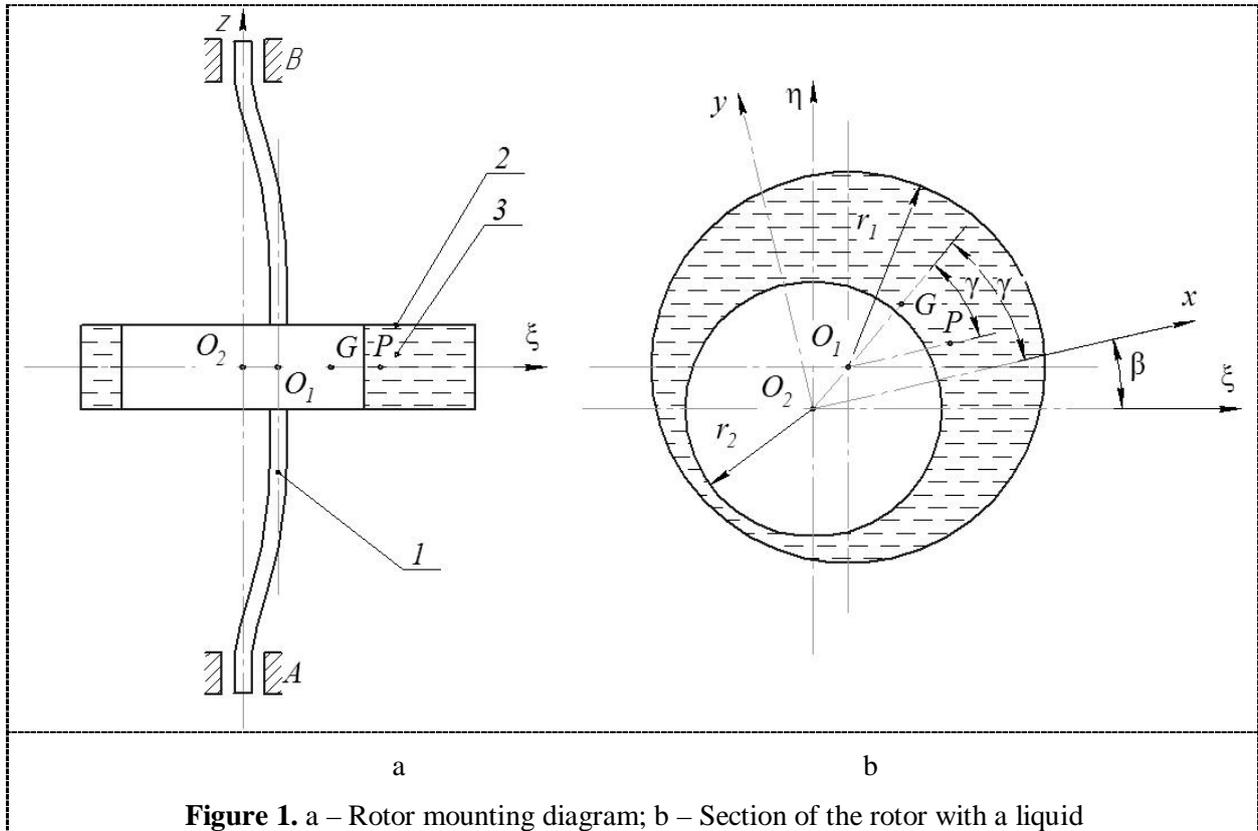
Figure 1. a – Rotor mounting diagram; b – Section of the rotor with a liquid
