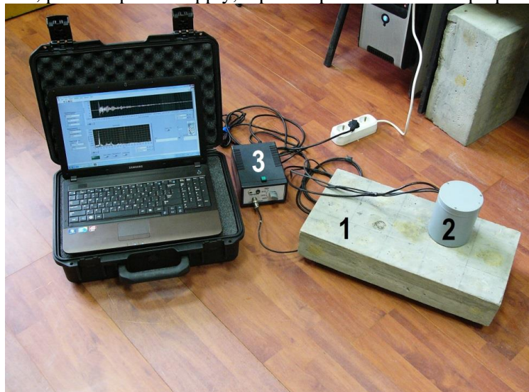
Figure 1. Laboratory complex: 1 – sample, 2 – external measure probe, 3 – portable power supply.
