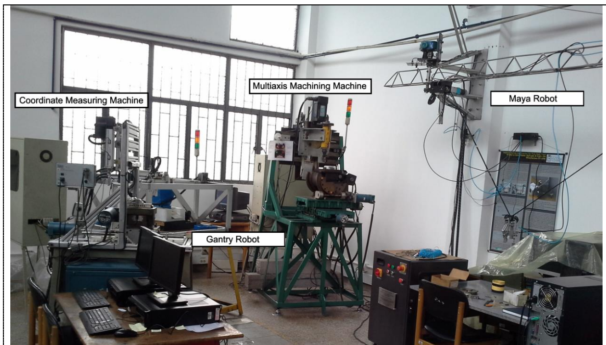
Figure 2. Experimental Manufacturing Cell's Machines and their physical disposition. Universidad Nacional de Colombia. Mechanics and Mechatronics Department. Cam-Mechatronics room Lab
