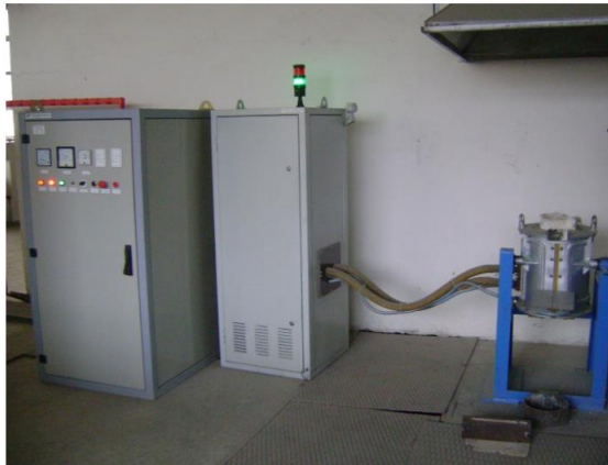
Figure 1. Induction heating furnace of medium frequency 8000 Hz.
