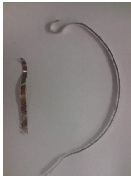
Fig. 1 specimen outlook before and after cold rolling indicating that the ribbon is elongated after the rolling [12]
