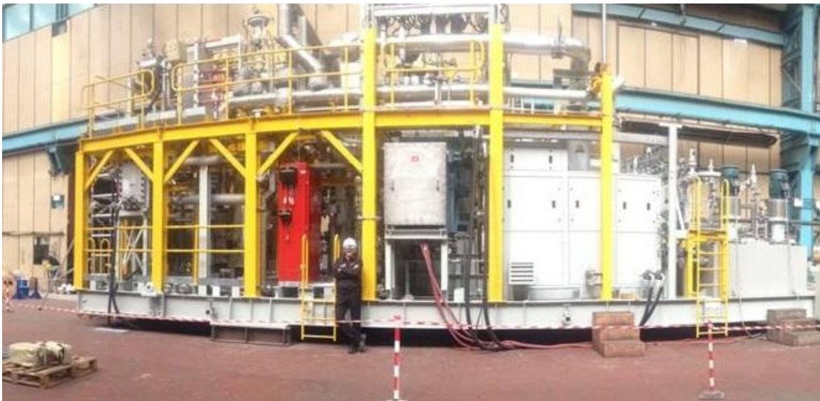
Figure 2: The compressor package on test with the author shown for scale reference
