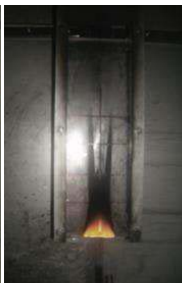
Figure 1. ULC specimen (Trial 1) during single-flame source test.
