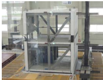
Figure 2. Make a seismic experiment Structure (Shaking Table)
