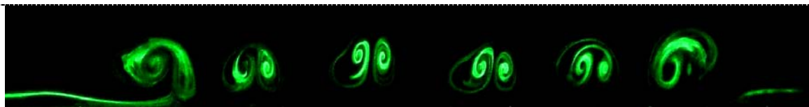
Figure 4. Counter-rotating Görtler type vortices with nearly uniform spanwise wavelength at the first peak of sinusoidal plate with the modified leading edge, Re = 3350 (taken from [30]).
