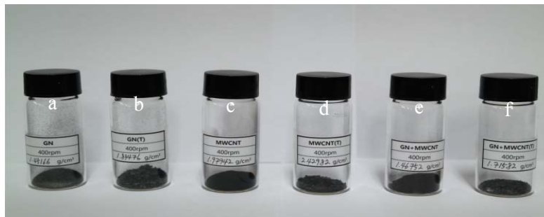
Figure 1. a) Dry ground GN, b) Wet ground and heat treated GN, c) Dry ground MWCNT, d) Wet ground and heat treated MWCNT, e) Dry ground GN-MWCNT, f) Wet ground and heat treated GN-MWCNT(T)
