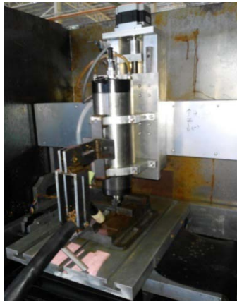
Figure 1. Mini CNC Machine with plasma torch attached in front of the spindle.
