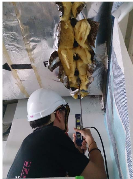
Figure 3. Measuring fresh air flow rate inside the ducting.
