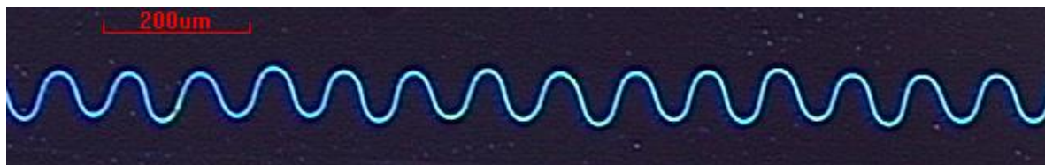
Figure 2. Optical images of the morphology of the serpentine microstructure.
