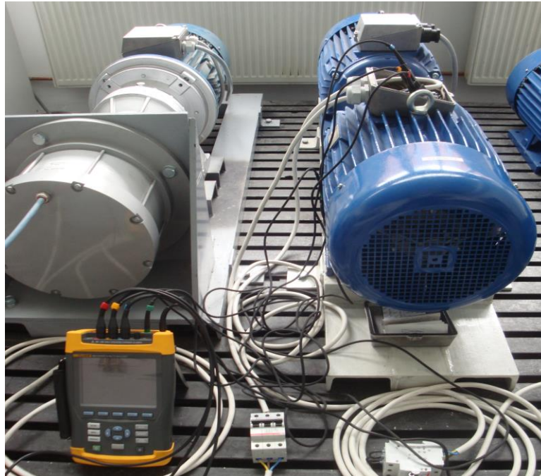
Figure 5. Generator DSWA coupled with prime mover induction motor under experimental tests.
