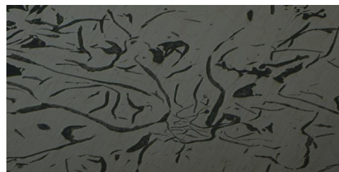
Figure 5. Metallographic examination for iron phosphorous.
