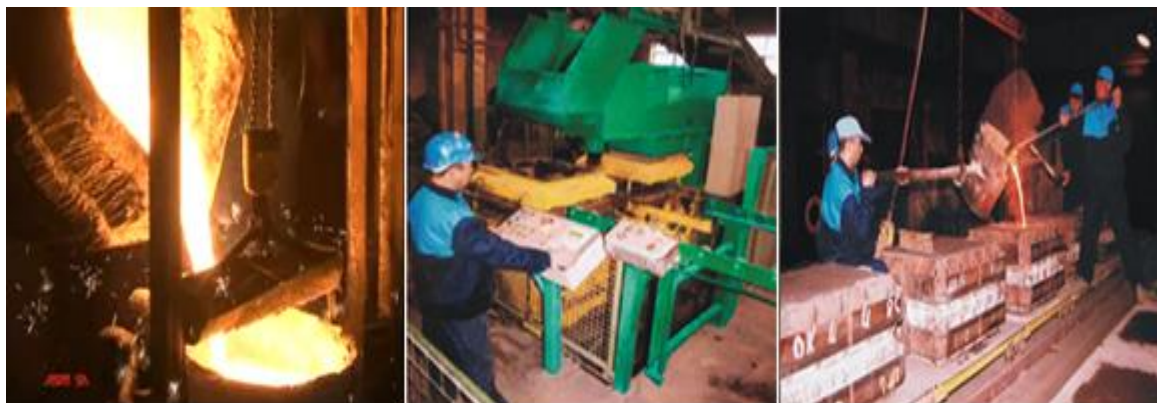
Figure 2. Flow technology for producing brake blocks.
