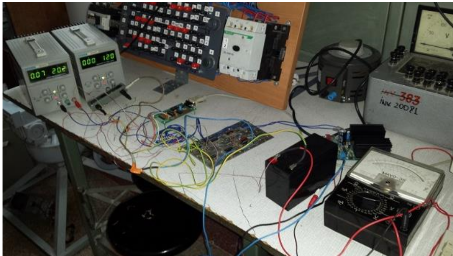
Figure 8. Overview from experimental setup with the lead acid battery (12 V, 9 Ah) charging from K 8012 source.
