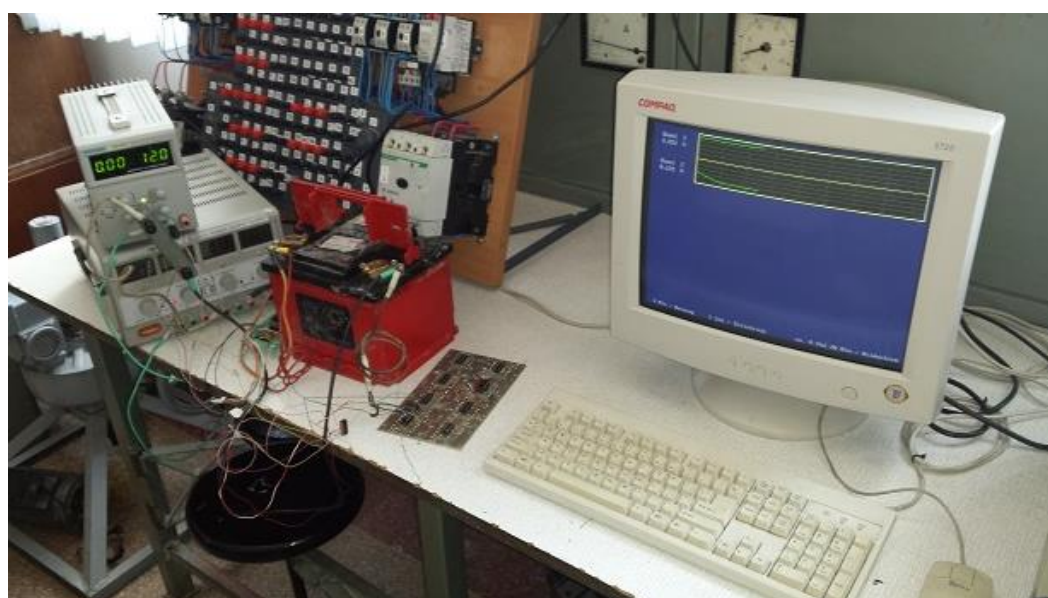
Figure 12. Overview from experimental setup with the lead acid battery (12 V, 47 Ah, 390 A) charging from power source AX 3003D-3.
