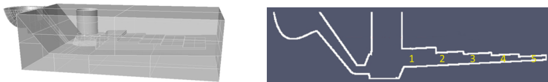
Figure 2. The gravity die and the 2D-model of the gravity die.
