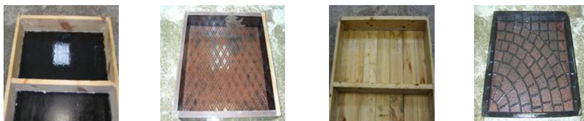
Figure 1. Formworks used for horizontal specimens
