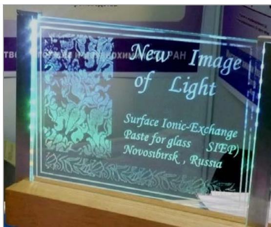
Figure 7. The glass sample decorated with the surface ion exchange paste (SIEP) and illuminated by coloured LEDs (a gold medal on the fair SIBPOLYTECH-2009, ITE Siberian Fair, Novosibirsk, Russia).
