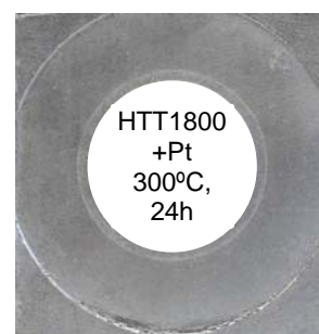
Figure 9. HTT1800 + Pt passivated foil after adhesion test
