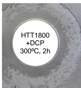
Figure 5. HTT1800 + DCP passivated foil after adhesion test
