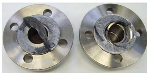
Figure 1. Example of adhesion of the graphite gasket on the stainless steel flange.
