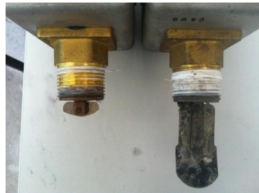
Figure 9. The lamella of the mechanical flow switch, respectively, after and before length modification made to avoid clogging risk.
