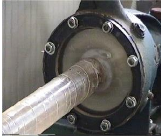
Figure 2 Pump working with two phase flow. Particular of the transparent flange
