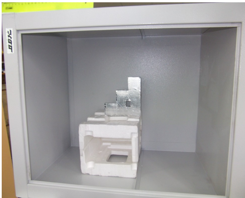
Figure 7. The test object inside the metal safe.
