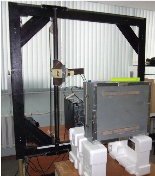
Figure 4. The UWB-scanner and the packing box.
