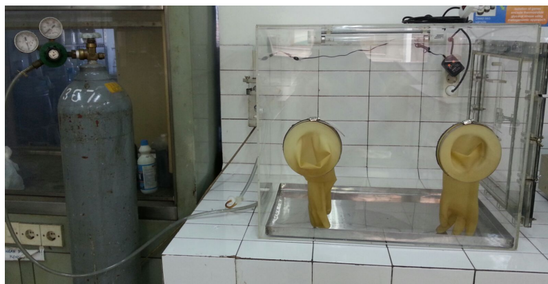
Figure 2. A simple anaerobic chamber connected with a nitrogen gas tube and equipped with a UV lamp.
