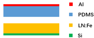
Figure 1. Structure of the triboelectric nanogenerator (TENG)
