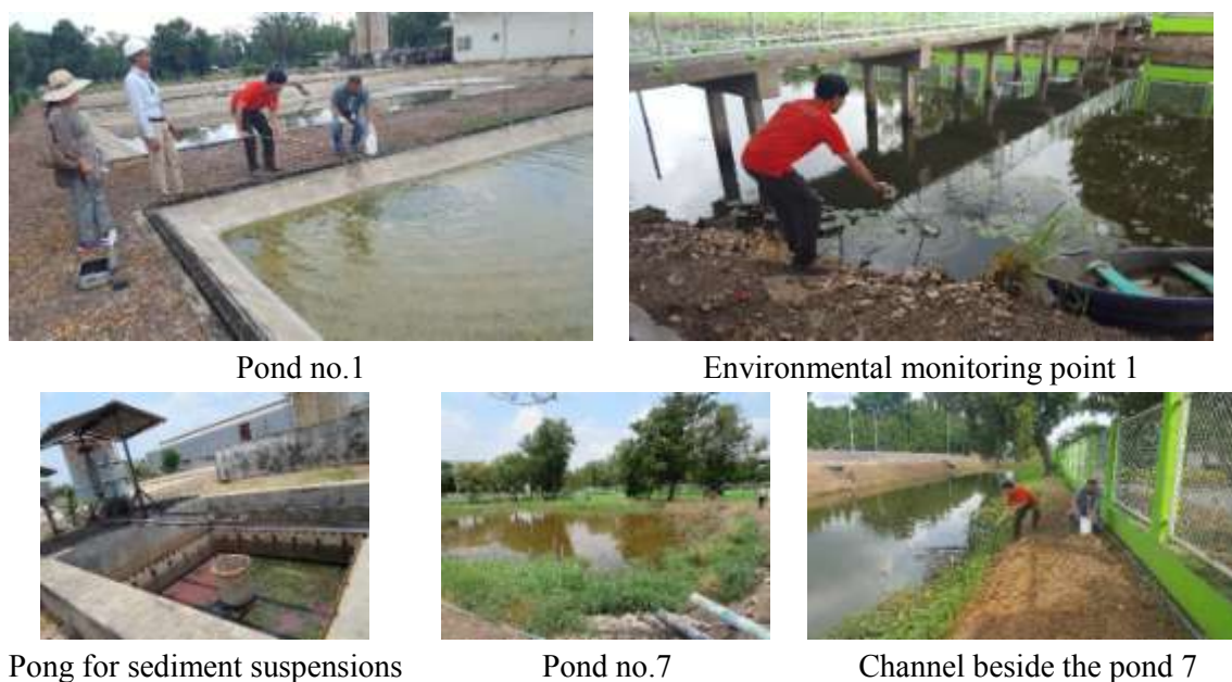
Figure 3. Sampling water samples from ponds onsite
