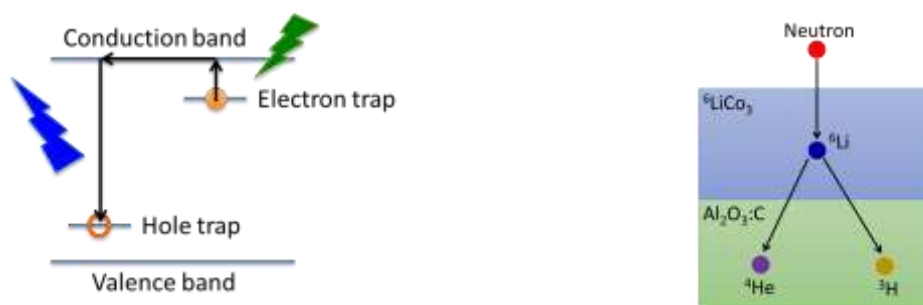
Figure 2. The OSL process (left) and the principle of albedo-type OSLN dosimeters.
