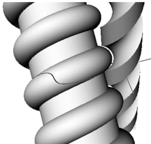
Figure 3. Superficial model of the contacting surfaces.
