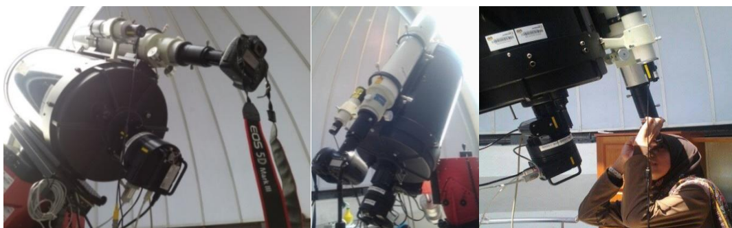
Figure 1. Instrumentation used for sunspot imaging with Camera EOS 5D mark III attached to Telescope Takahashi FS-102 NSV at National Planetarium, Kuala Lumpur.
