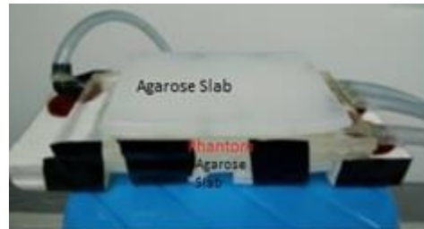
Figure 4. The agarose gel slabs placed on the top and bottom of the fabricated phantom.
