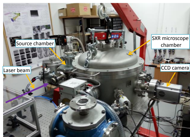
Figure 1. Photograph of the SXR microscope.
