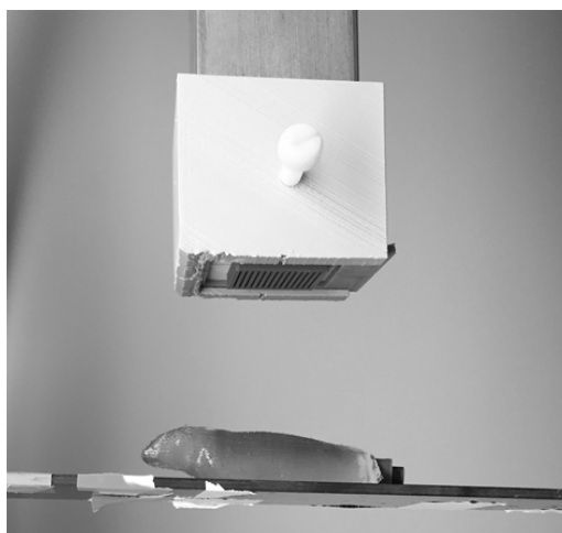
Figure 1. Rodent-morphic Presage dosimeter set-up in X-Rad irradiator with radiation grid block mounted to collimator.
