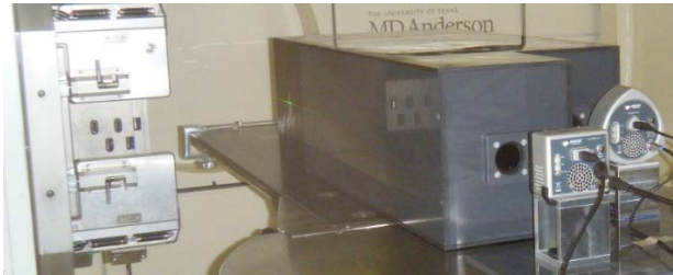
Figure 1. The large-volume liquid scintillator detector, including the tank and two cameras, in position on the patient couch of the Proton Therapy Center - Houston scanning gantry.
