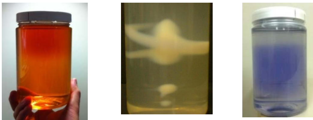
Figure 1. A recent illustration of the 3D dose information captured in three different gel dosimeters from the proceedings of IC3Ddose [21]. (left) The Fricke-xylene-orange-gelatin dosimeter shows a colour change in the volume irradiated with a 12 MeV electron beams. (centre) The polyacrylamide polymer gel dosimeter shows increased scatter in the high dose areas radiated using a Cobalt-60 tomotherapy IMRT delivery. (right) The colour change of a Leuco-crystal-violet micelle gel dosimeter after a VMAT prostate plan irradiation.
