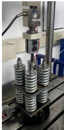
Figure 7. Butt welded specimen in the axial fatigue equipment.
