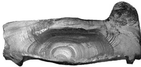
Figure 1. Fracture surface of the broken train wheel [1].
